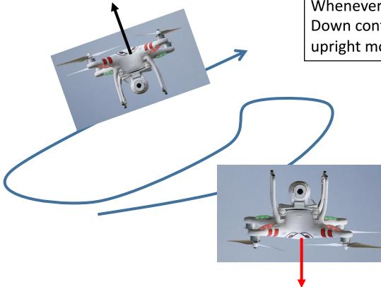
Whenever the UAV reaches an Upside-Down configuration, it must reach an upright mode within 2 seconds.
